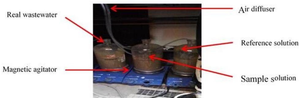
**Fig. 1. Biological treatment device using the ZW method**
