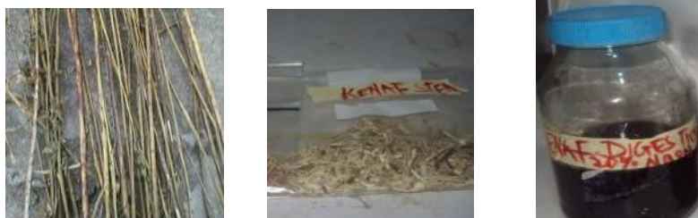
Fig. 1. Kenaf stem Shredded stem Pulping effluent
